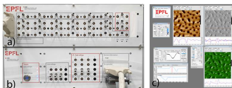
Figure 1: Open source SPM controller consists of an FPGA-based modular controller electronics (a), a high voltage amplifier (b), a software suite with the real-time controller and the user interface (c).
